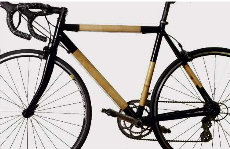
'Aluboo' (bamboo alloy) bicycle frame made by James Wolf of Boo Bicycles.
