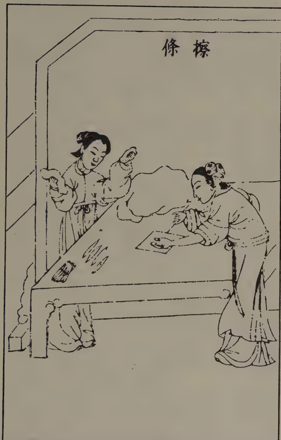
Figure 2-17. Straightening and rolling bowed cotton fibers into long slivers with the aid of wooden boards.
