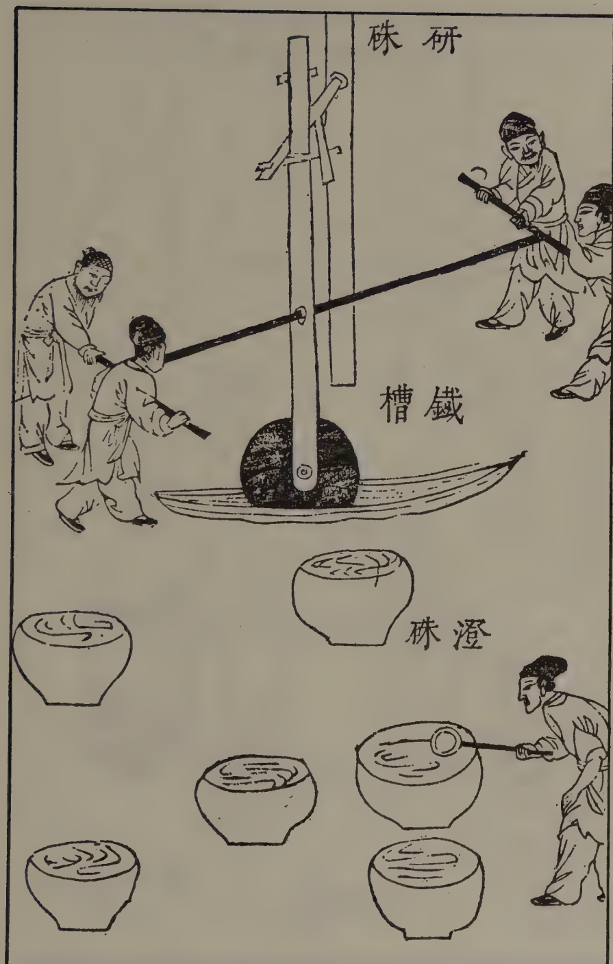
Figure 16-1. Grinding and hydraulic classification of mercury ore.
