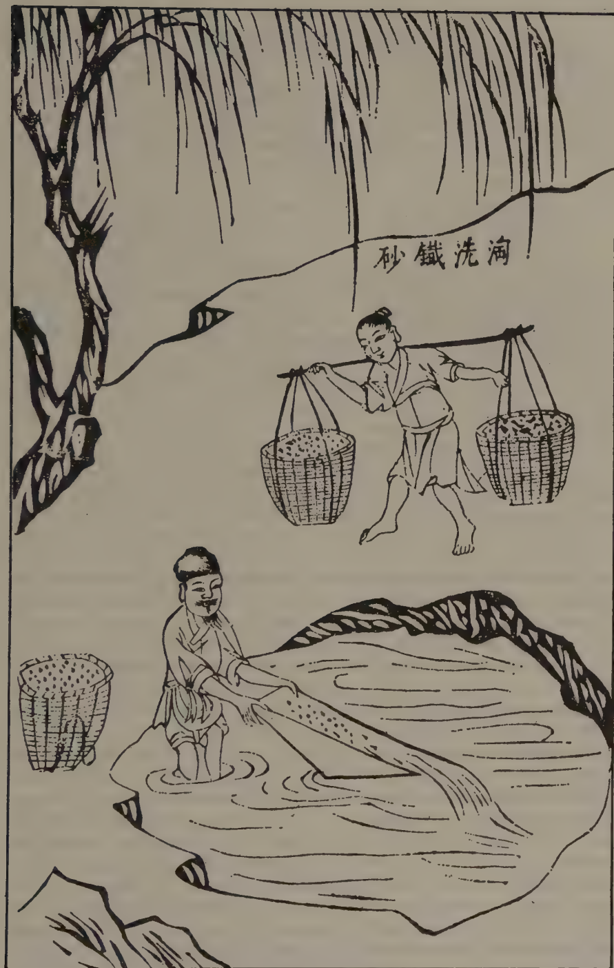
Figure 14-9. Concentrating iron ore by washing.
