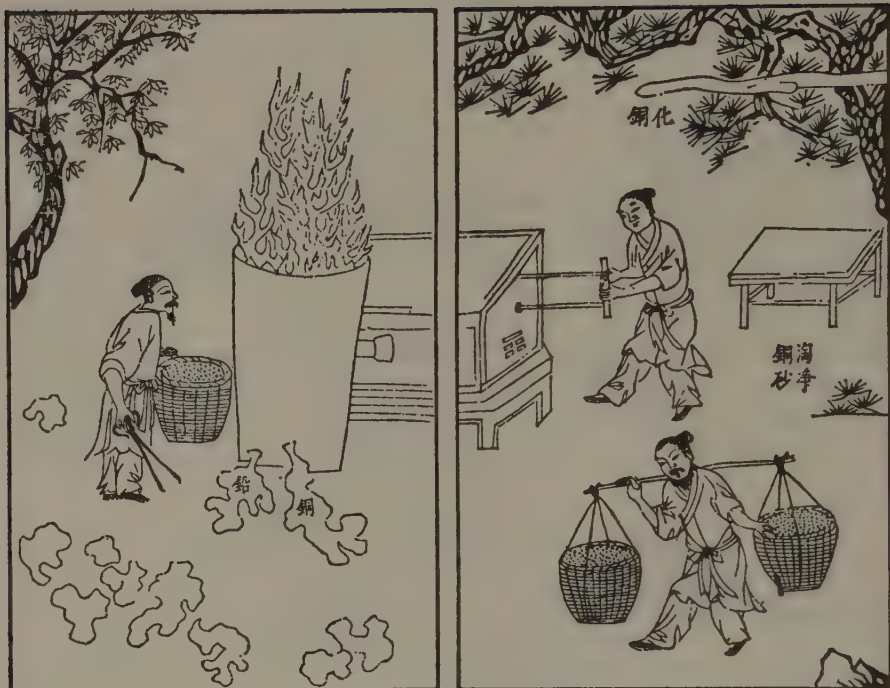
Figure 14-6. Smelting an ore containing both copper and lead; molten lead and copper flowing out from two separate holes.
