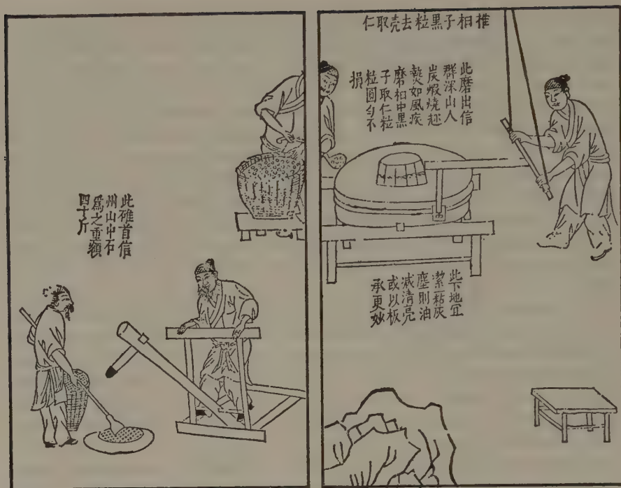
Figure 12-3. Pounding (left) and grinding (right) vegetable tallow tree seeds.
