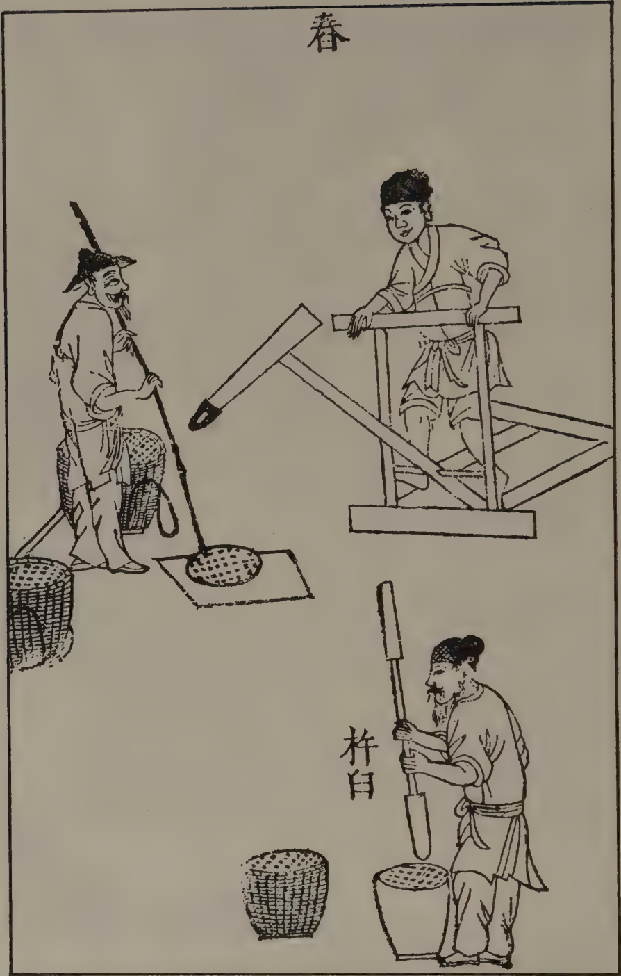
Figure 4-11. Hand- and foot-operated pounding mills.
