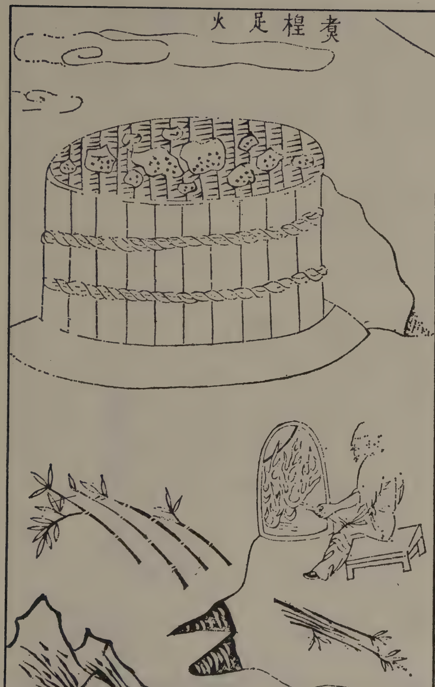
Figure 13-2. Cooking the inner mass of bamboo in a pot.
