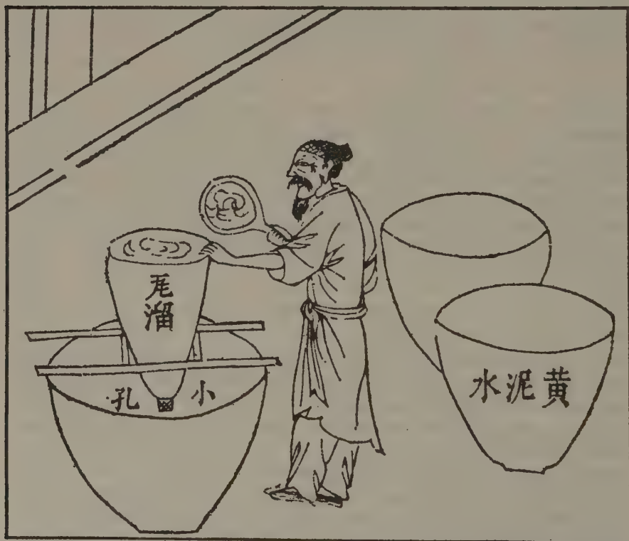
Figure 6-2. Removing dark impurities from crystallized raw sugar.
