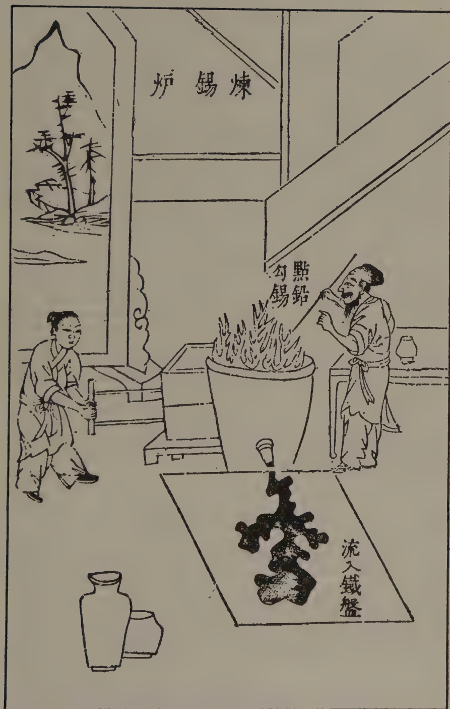
Figure 14-13. Smelting tin ore with the addition of lead.
