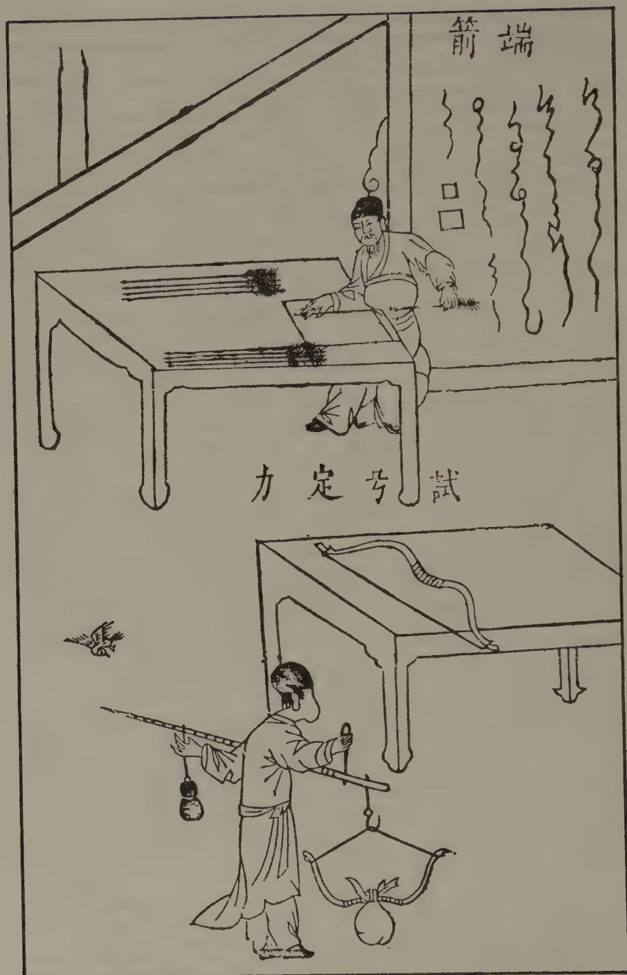
Figure 15-1. Straightening the shaft of an arrow (top) and determining the weight or pull of a bow (bottom).
