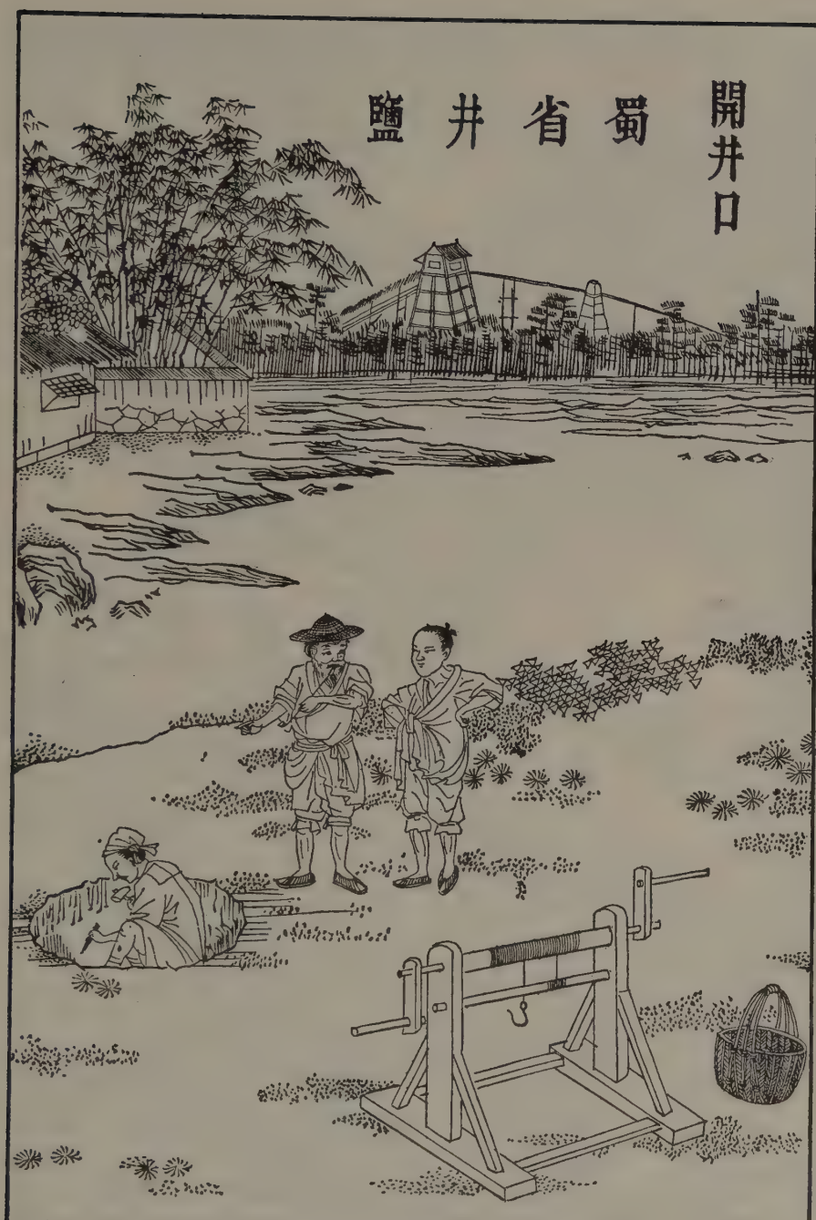
Figure 5-6. Opening ground for drilling a salt well [Ch'ing addition].
