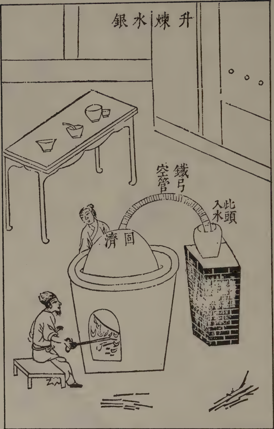
Figure 16-2. Sublimation and condensation of mercury ore.
