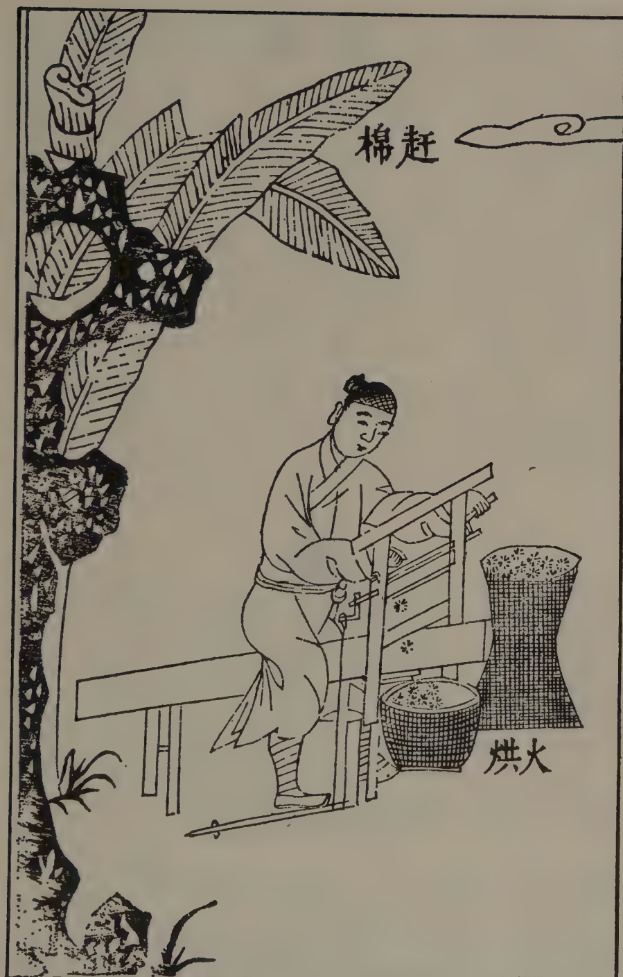
Figure 2-15. A cotton gin for separating fibers from seeds.
