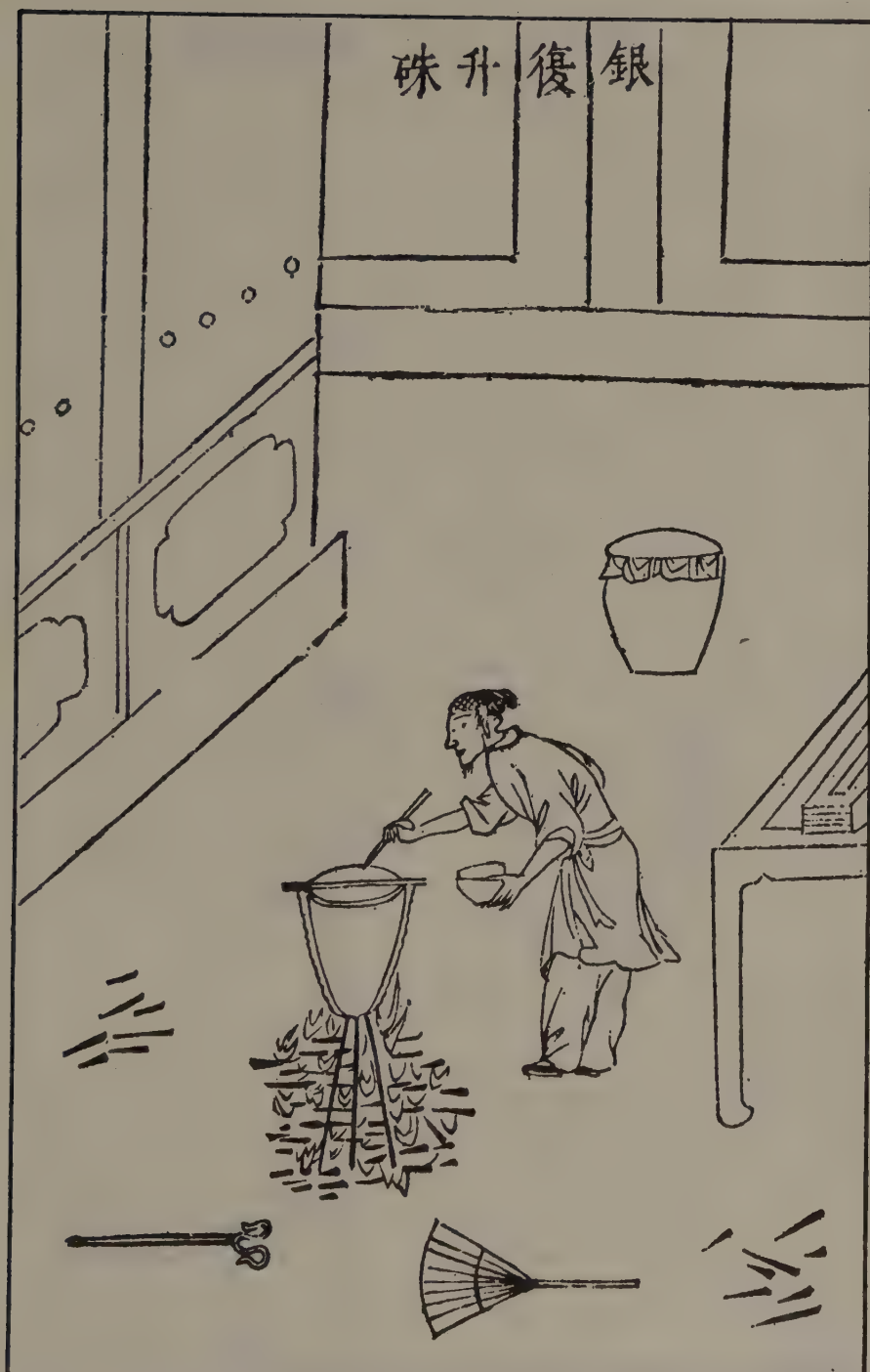
Figure 16-3. Making vermillion through sublimation of mercury with sulphur.
