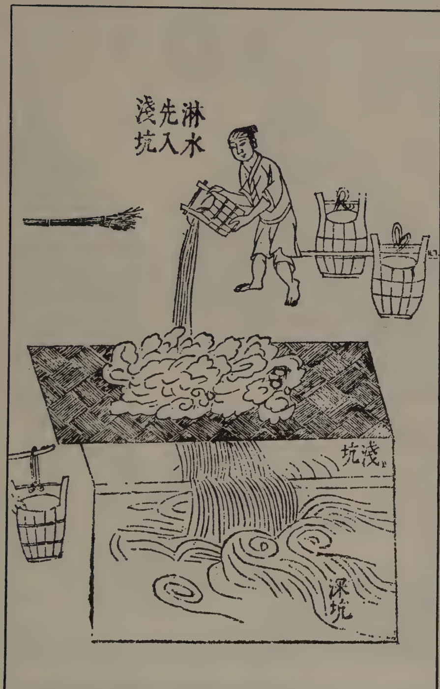
Figure 5-2. Sea brine passed through raw salt in a reed mat and allowed to drain into a shallow pit.
