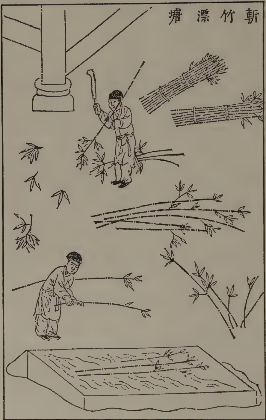
Figure 13-1. Steeping and washing cut bamboo.
