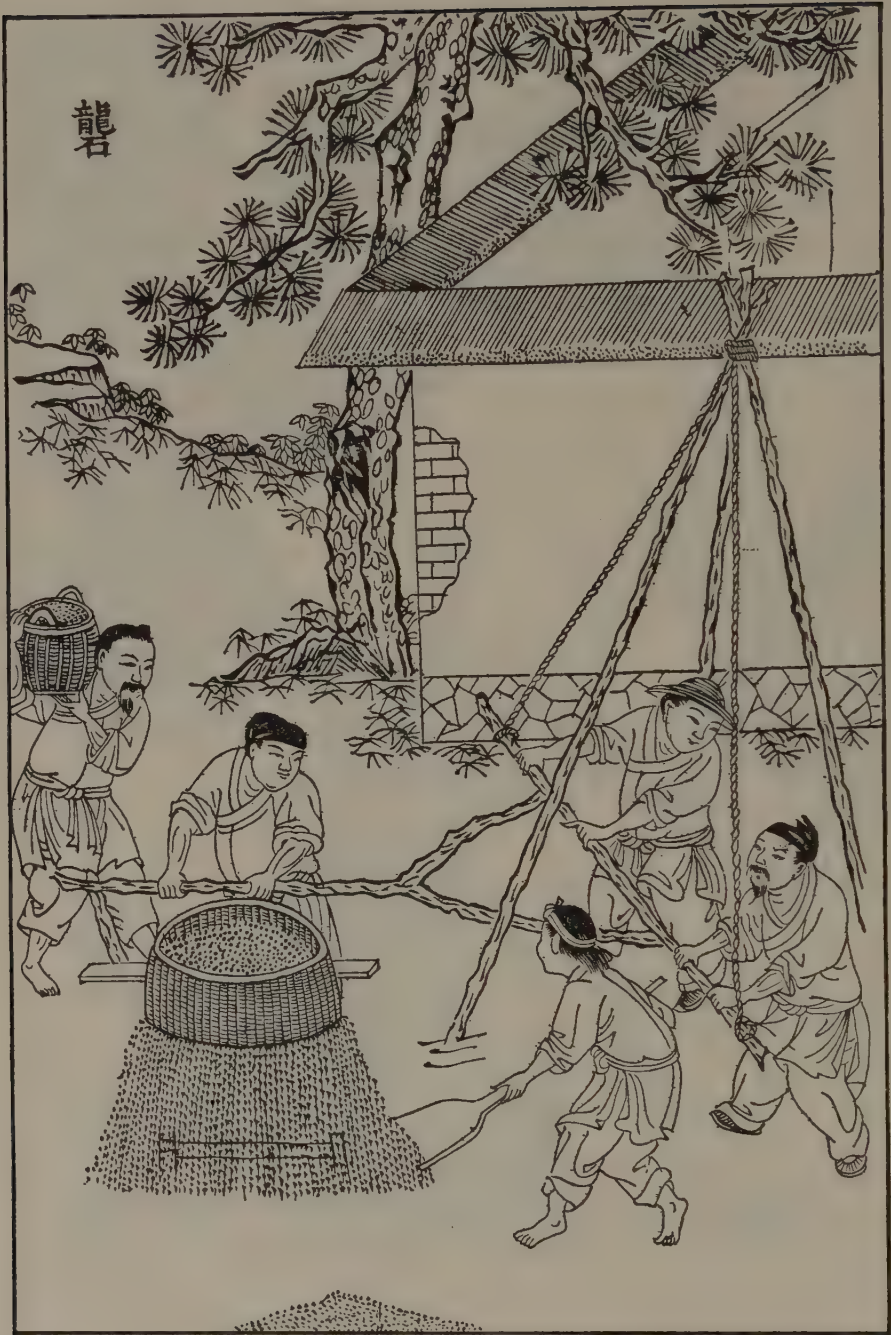
Figure 4-9. Unhusked grains being sieved out and returned to the hulling mill [Ch'ing addition].
