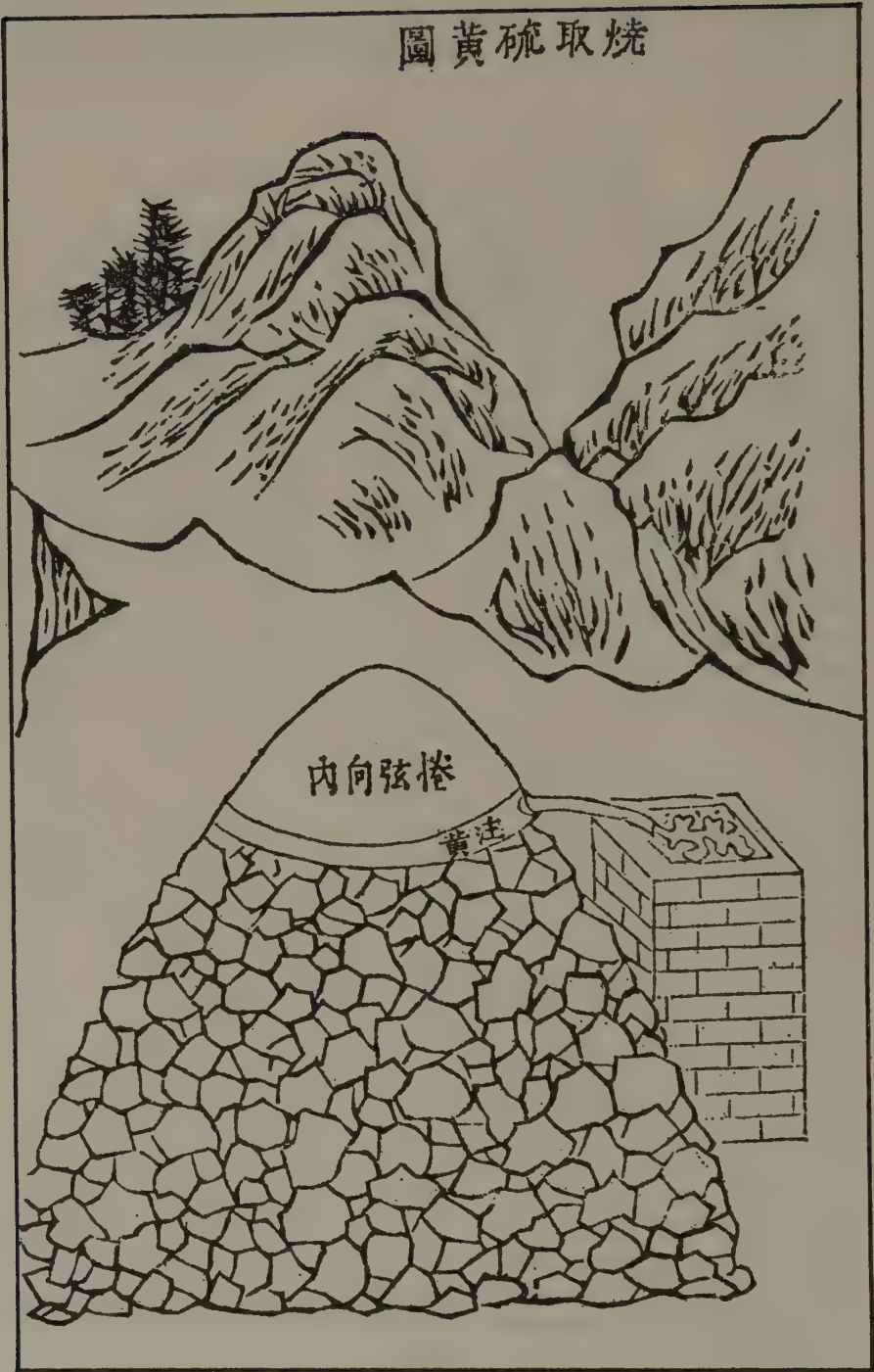
Figure 11-5. Calcination of pyritic stones for sulphur.
