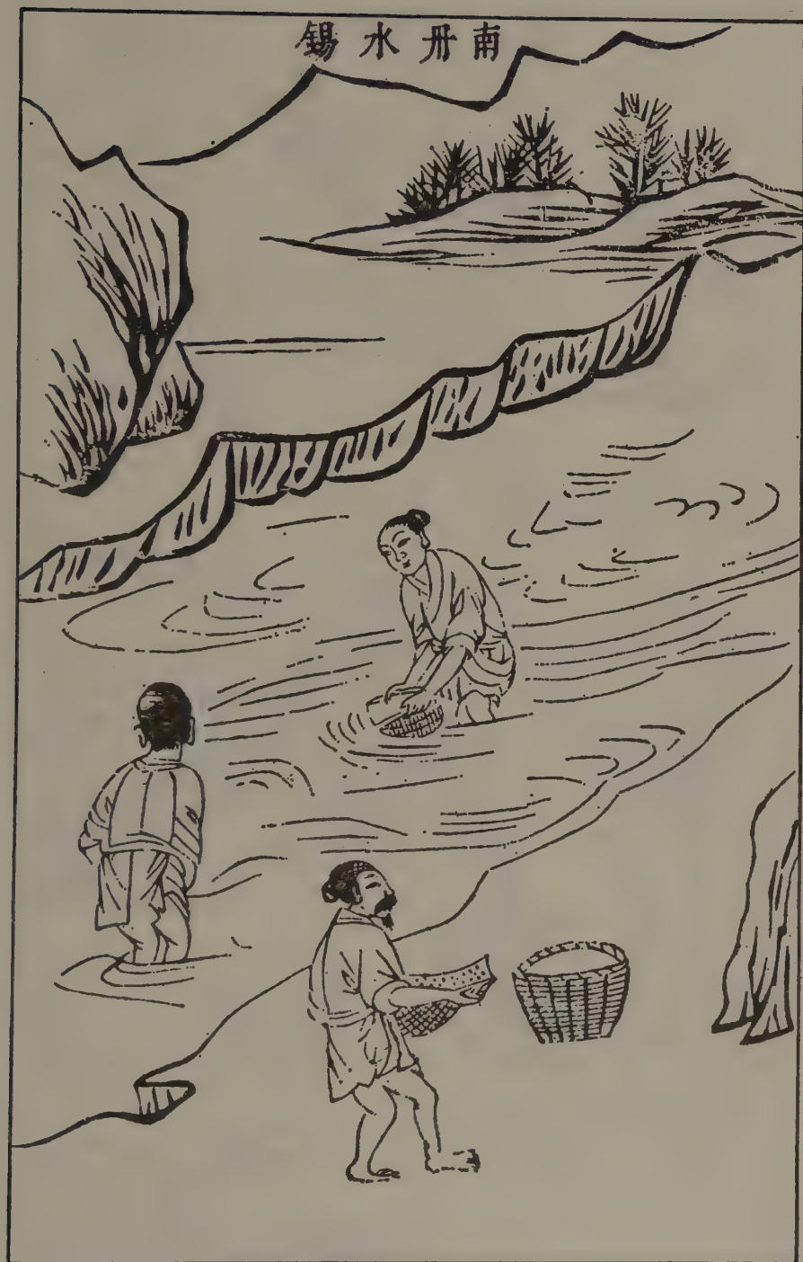
Figure 14-11. Recovering tin ore from the river at Nan-tan, Kwangsi.
