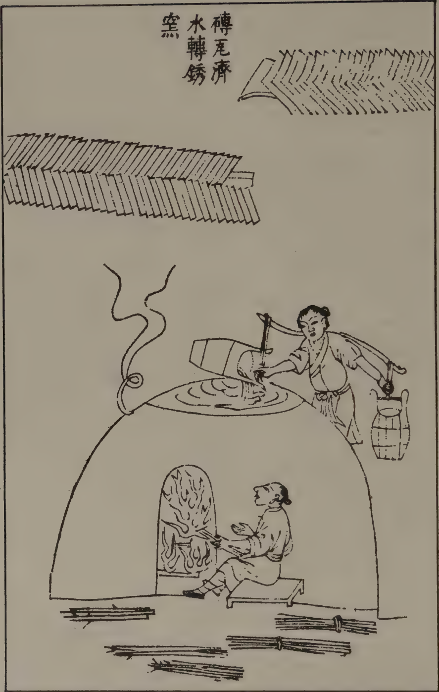
Figure 7-3. Superficial glazing of bricks and tiles by water-quenching.
