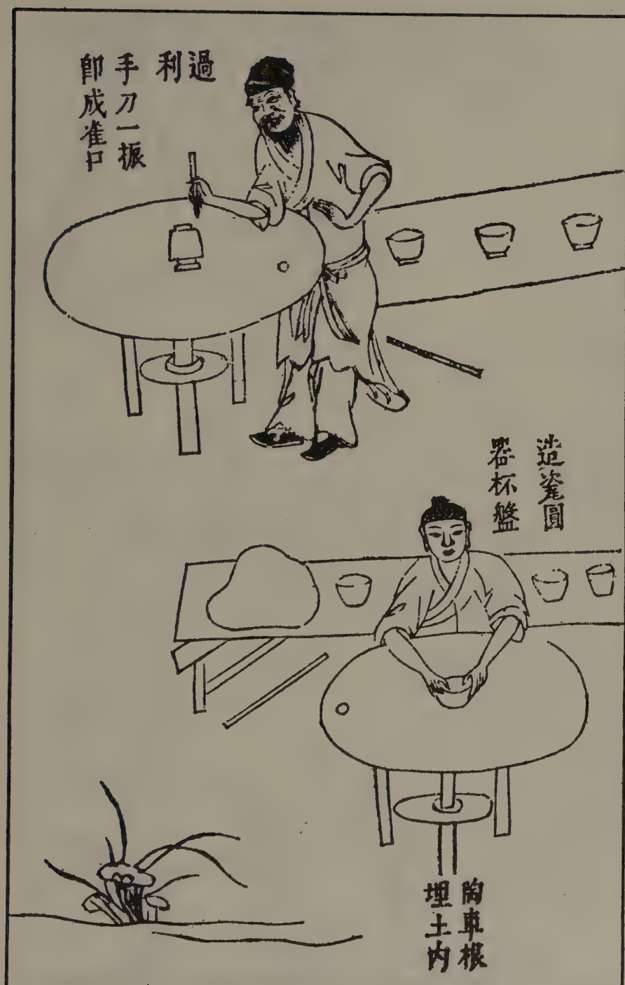
Figure 7-8. Shaping (lower) and polishing (upper) clayware with potter's wheel.
