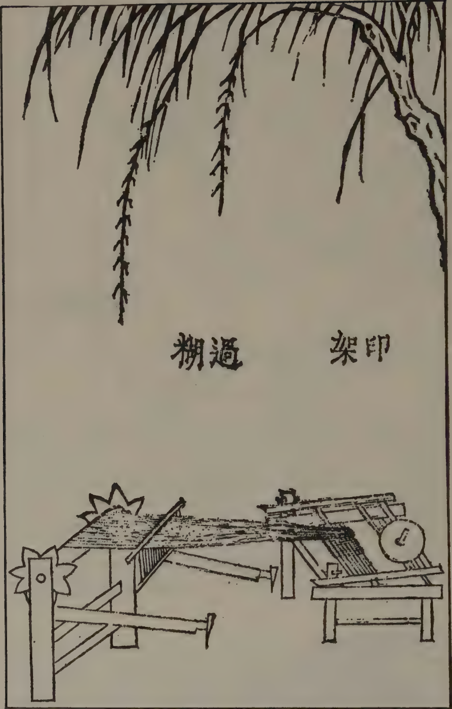
Figure 2-12. A warp frame for separating and sizing warp threads.
