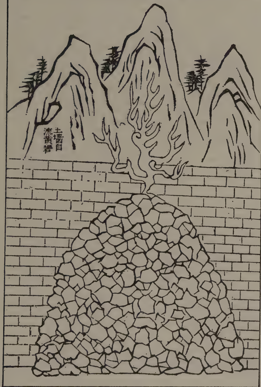
Figure 11-4. Burning copper coal for black vitriol.
